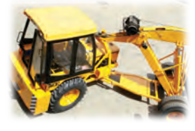
9 TURNING RADIUS Lower turning radius of 5.5 mtrs. facilitates better maneuverability and movement in confined spaces.
